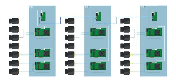
C2C-Link is able to accurately synchronize cameras that are connected to the same frame grabber, or to different frame grabbers in the same PC, or even to different frame grabbers in different PCs. The synchronization is managed through a master/slave architecture. The master board receives all trigger signals and propagates them to slave boards, ensuring that all cameras are acquiring lines at the exact same time.
