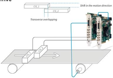
When several CIS are required to cover the whole area to be inspected, they are usually staggered. The reason is to avoid losing pixels between CIS that are placed side by side.
